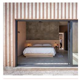
ABOVE: Large sliding windows provide entry to the interiors, where the ribbed concrete surfaces are ontinued and blended with smooth walls and wood furnishings. The exteriors' fluted surface creates shadows that help keep the interiors cool.
